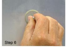
Push part into the substrate to squeeze adhesive out from base.
