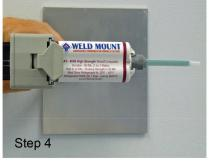
Fit tip onto CL-AT-8040 cartridge.
